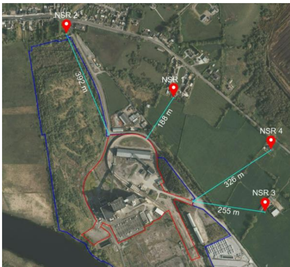
Figure 4.7: Nearby Sensitive Receptor (NSR) Locations and Site Layout
